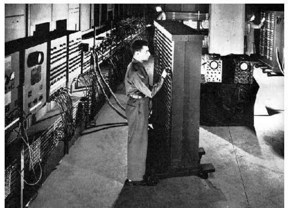
First High-Speed, General Purpose Computer Using Vacuum Tubes: Electronic Numerical Integrator and Computer (ENIAC)
