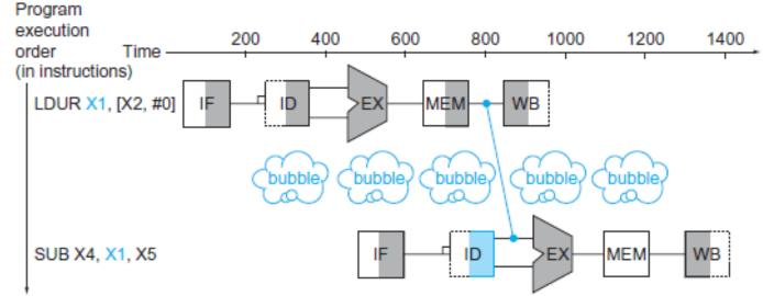
Here we must insert a stall, to allow X1 to be used in the SUB instruction.
