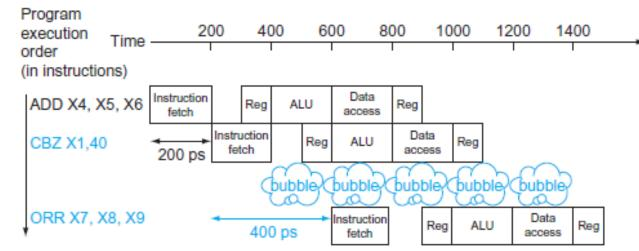
This however introduces additional delay into the pipeline.
