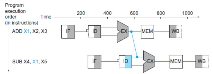
Forwarding is the addition of extra hardware allowing us to bypass some stages and access the interim result.
