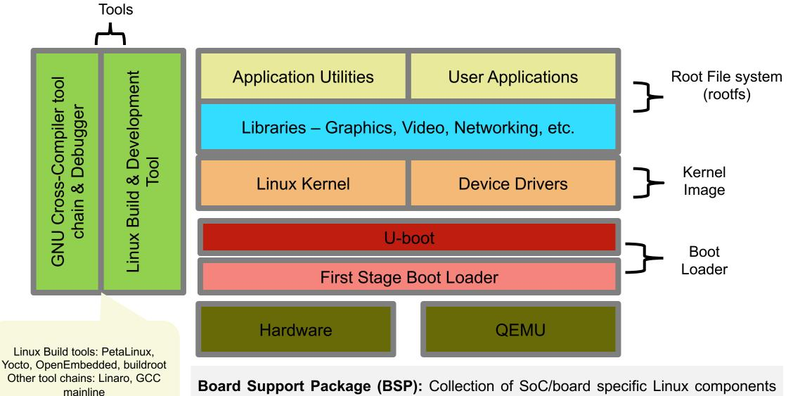
that include Linux kernel & device drivers, boot loader and tools
