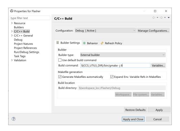
**Step 5**: Expand the C/C++ tab and then select "Build Variables". Add the variable "CCS\_UTILS\_DIR and paste in the directory of CCS\utils. Then "Apply and Close". Again, your version of CCS may be not be ccs1260.
