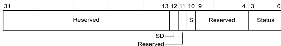
Figure 3-31 Instruction Fault Status Register format
