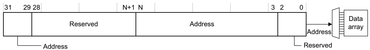
Figure 3-88 L2 data RAM array read operation format
