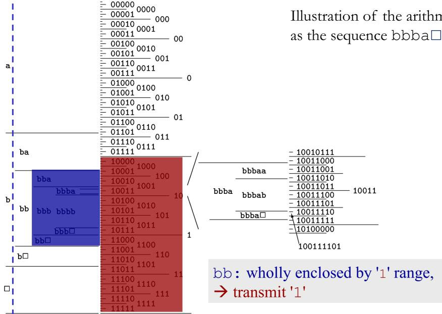
Illustration of the arithmetic coding process as the sequence  $bbba\Box$  is transmitted
