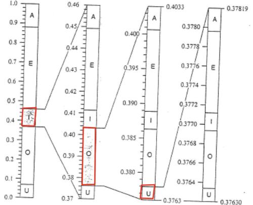
To send "iou": Send any interval C within [0.37630, 0.37819) Using a binary fraction of 0.011000001 (9 bits) (It would be 10 bits in Huffman coding)
