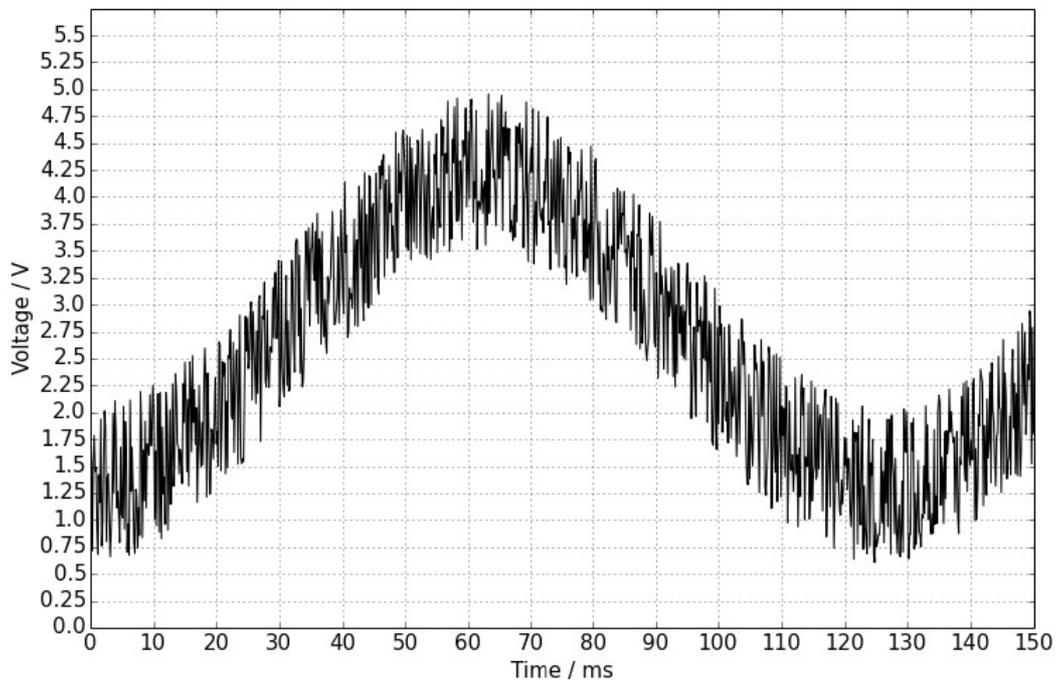
(ii) The image above shows a signal produced by an IR sensor. Sketch (on the image) what the same signal would look like once it had been stored on the RPi (i.e. once it has been digitized by the ADC) if the ADC was 2-bit and sampled every 10 ms. Label your diagram so that each change from the original signal is clearly explained.
